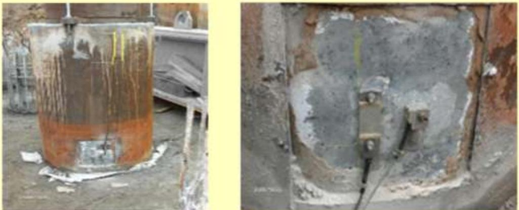
**Pile head prepared for dynamic load test Sensors installed on the pile head**
